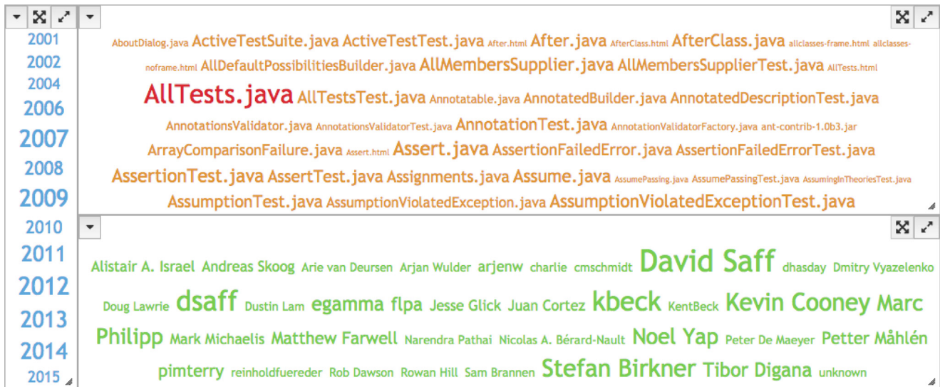
Fig. 2. Multiple linked tag clouds of the JUnit Repository in ConceptCloud, showing changed files (top), authors (bottom) and years (left). The tag cloud is constructed from a revision-based context.
